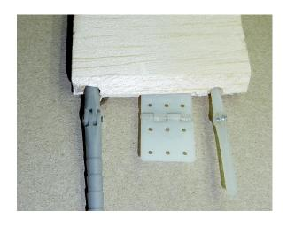
I used the usual, but not excessive, care applying the glue. Using a toothpick I poked some into the holes and slots and put a little on one side of the flat hinge and the bodies of the round ones. I wiped the wood surface with meths before inserting the hinges. I did the V-shaped side of the joint first and allowed the 15 minute glue to cure for an hour. There
